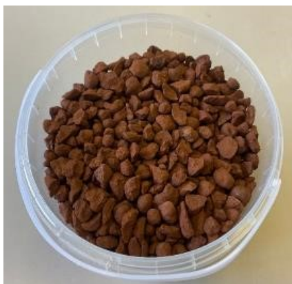
Initial sintering RM from the APC-layer complex.
